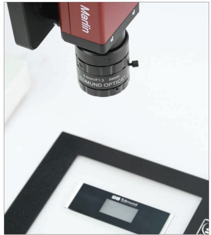
Ronchi Ruling Comparison Test Setup
